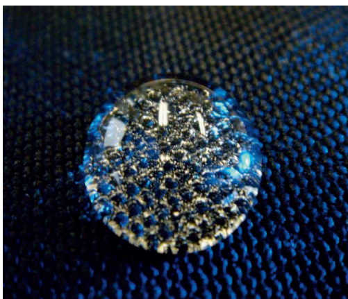
Oil drop on a nano-impregnated fibre
