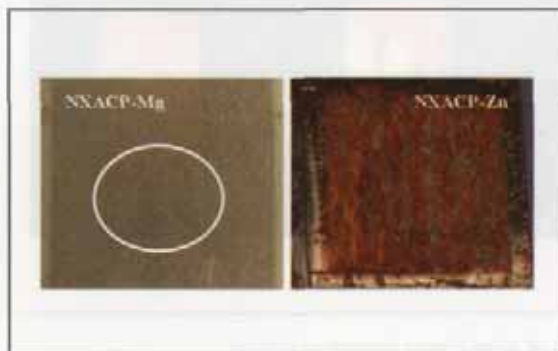
Figure 3: Comparison of 22MnBS steel plates with 7 \mu\text{m} coating after treatment for 200 h at 600 °C and 100 hr salt spray test; left: NXACP-Mg; right: NXACP-Zn
